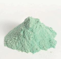
DIPSORB powders are approved by the CEDRE (French documentation, research and experiment center for accidentally polluted waters). They have oleophilic properties and are used in the absorption of oils and hydrocarbons. They come in packs, cushions or mattresses to facilitate their use.
